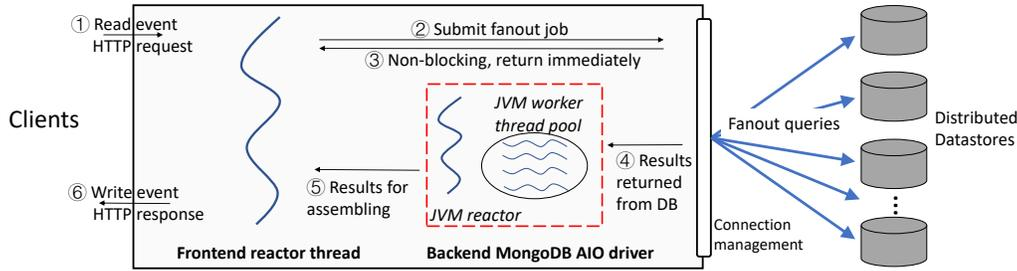
Figure 6. Architecture of the asynchronous AIOBackend server.
