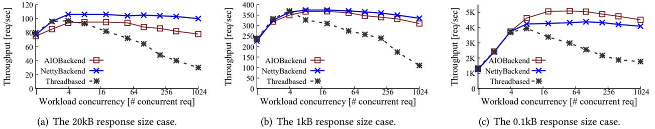
**Figure 5. Throughput comparison among different drivers for MongoDB under different workload concurrencies and fanout query response sizes.** The fanout factor is fixed to 5. Subfigures (a) and (c) show that the throughput order between AIOBackend and NettyBackend is reversed when the fanout query response size changes.
