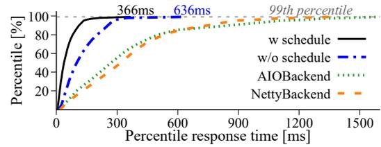
**Figure 16. Percentile response time comparison among different servers running on the YCSB dataset with large data shard size** (i.e.,  $\times 10$  times the size of that in Figure 15(a)). The fanout factor of *Lfan* and *Sfan* requests is 5 and 3. DoubleFaceNetty with scheduling still outperforms the other three cases in tail latency.
