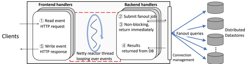
**Figure 10. Architecture of DoubleFaceNetty.** One (or a few) reactor thread is (are) responsible for managing both the events from the upstream clients (e.g., HTTP requests) and from the downstream datastores (e.g., fanout query responses).
