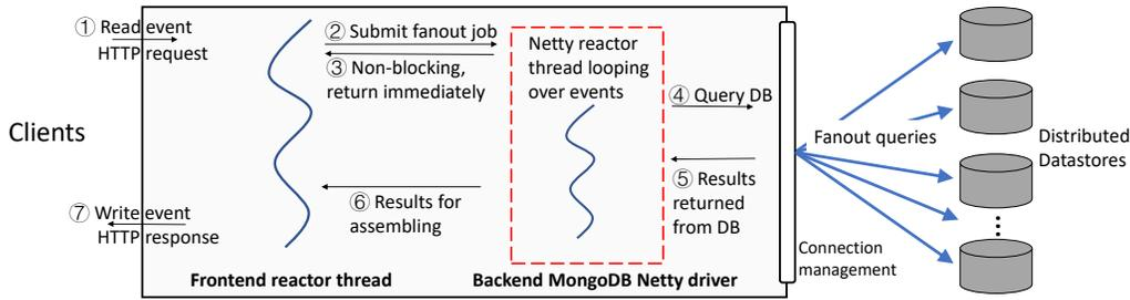
Figure 8. Architecture of the asynchronous NettyBackend server.
