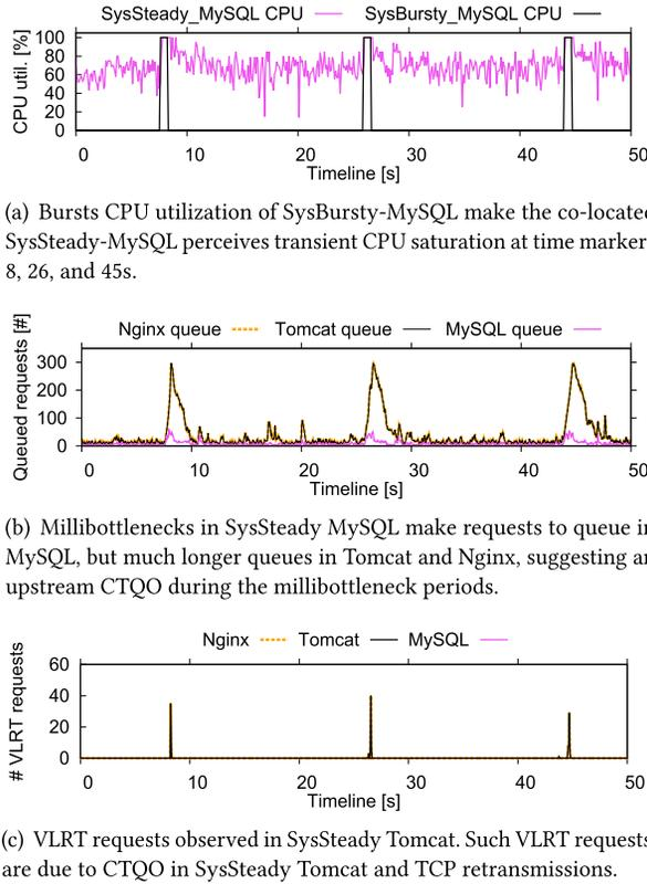
Fig. 10.  $NX=1$ , Nginx-Tomcat-MySQL configuration when millibottlenecks occur in MySQL. Upstream CTQO observed between MySQL and Tomcat during the millibottleneck periods.
