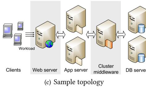
Fig. 1. Experimental setup of the VMware ESXi cluster.
