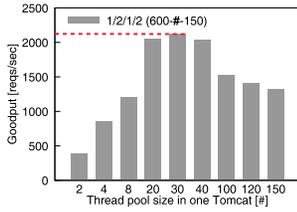
(a) Validation of thread pool size in Tomcat. 30 is recommended under the 1/2/1/2 hardware configuration.
