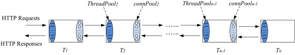
Fig. 11. A simple model of  $n$ -tier applications with soft resources. Except the last tier (database tier), every server has a thread pool to process incoming requests and a connection pool to communicate with the consecutive downstream tier.
