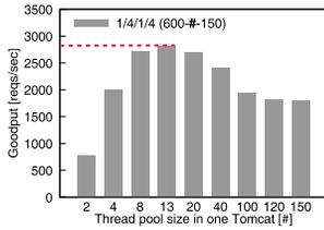
(d) Validation of thread pool size in Tomcat. 13 is recommended under the 1/4/1/4 hardware configuration.
