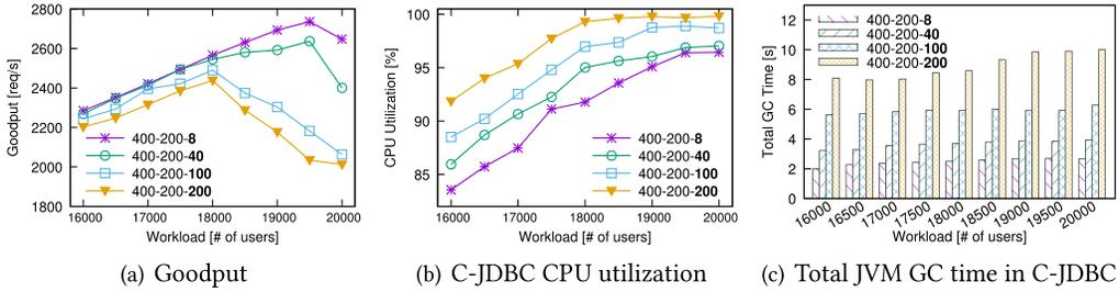
Fig. 5. Performance degradation caused by Tomcat DB connection pool over-allocation. The hardware configuration is 1/4/1/4.
