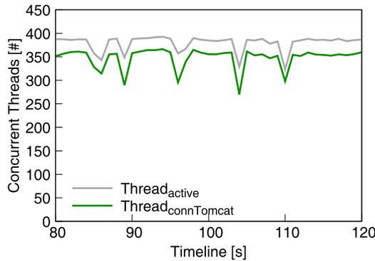
Fig. 8. # of Apache threads in connecting Tomcat among the total active Apache threads in the 400-6-200 case at workload 19,500. Four hundred threads in the Apache server enable a high number of Apache threads in connecting Tomcat, allowing a high number of concurrent requests to downstream tiers.
