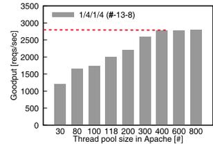
(f) Validation of buffering effect of Apache threads. 118 is recommended. But 400 is needed for highest goodput.
